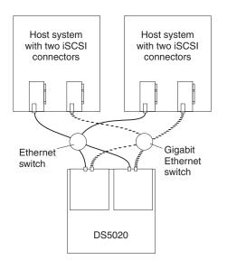
Figure 62. Example of a multiple-host, multiple-port configuration
